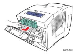
**3.** Pull the jammed paper slowly out of the printer. Verify that any torn pieces of paper are removed.
