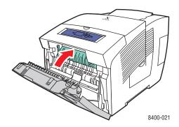
**6.** Insert the tray into the tray slot and push it completely to the back of the printer.
