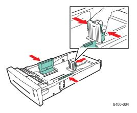
**4.** Remove jammed paper inside the printer tray slot. Confirm that any torn pieces of paper are removed.
