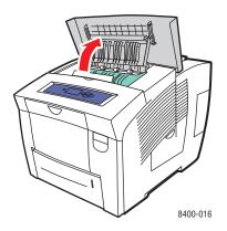
**2.** Pull the jammed paper slowly out of the printer. Verify that any torn pieces of paper are removed.
