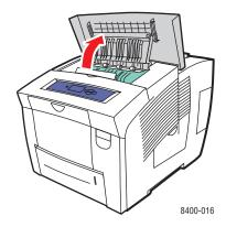
**b.** Pull the jammed paper slowly out of the printer. Verify that any torn pieces of paper are removed.
