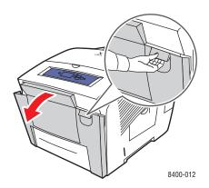
**b.** Pull the jammed paper slowly out of the printer. Verify that any torn pieces of paper are removed.
